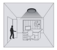
When ambient light is lower than the preset light threshold value, the sensor detects a temperature moving object, the lamp lights up automatically.
