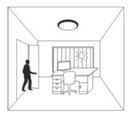
When the ambient light is bright enough, even if you detect a temperature moving object, lights don't come on automatically.
