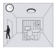
In the delay time, the sensor doesn't detect any temperature moving objects, the lights are off automatically.
