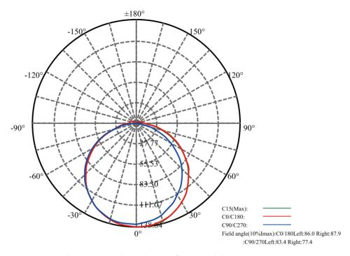
Beam Angle(50%Imax):C0/180Left:58.2 Right:60.4 :C90/270Left:60.6 Right:54.0
