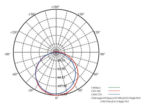
Beam Angle(50%Imax):C0/180Left:56.8 Right:60.7 :C90/270Left:58.9 Right:55.5
