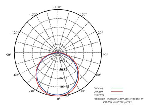
Beam Angle(50%Imax):C0/180Left:60.3 Right:57.3 :C90/270Left:59.0 Right:54.8
